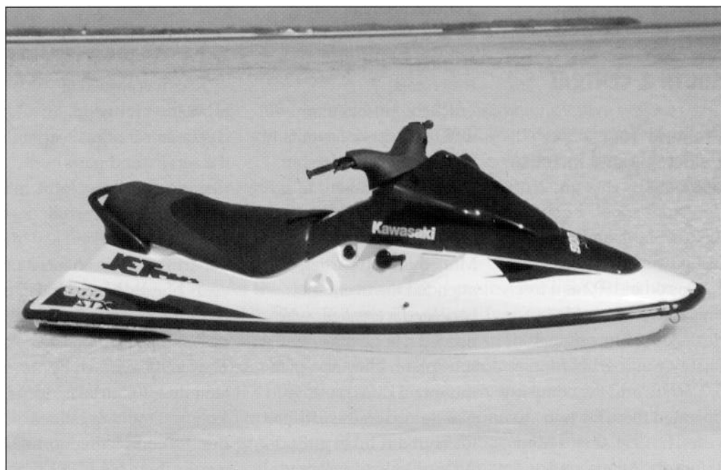
A revised STS hull and 900 ZXi powertrain are blended to create the 900 STX. Notice the service access hatch below the front corner of the seat.
