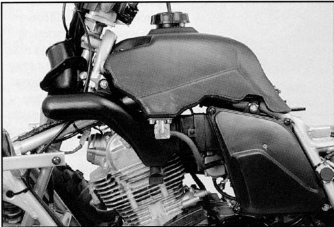
(ABOVE) Engine is adapted from Bayou 300 but has a different cam. (BELOW) Chain final drive is lighter than shaft and works well with Lakota's long-travel suspension.
