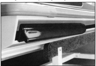
exit nozzle does not need mounting bosses for the nozzle trim pivot points. Because of this, the exit nozzle from the JS750SX is used. A quick-turn steering nozzle incorporating a vertical vane for more responsive cornering completes the XiR pump. The XiR generates 675 pounds of thrust.
