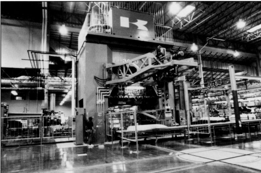
(ABOVE) Custom-made press for producing watercraft hulls has a 3,000-ton capacity! (BELOW) Superior-quality wheels emerge from an intricate process.
