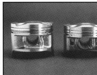
Lighter and stronger: "E" parts on the right vs. "D" parts on the left (photos clockwise from top left): valves, exhaust tappets, pistons and piston pins.
