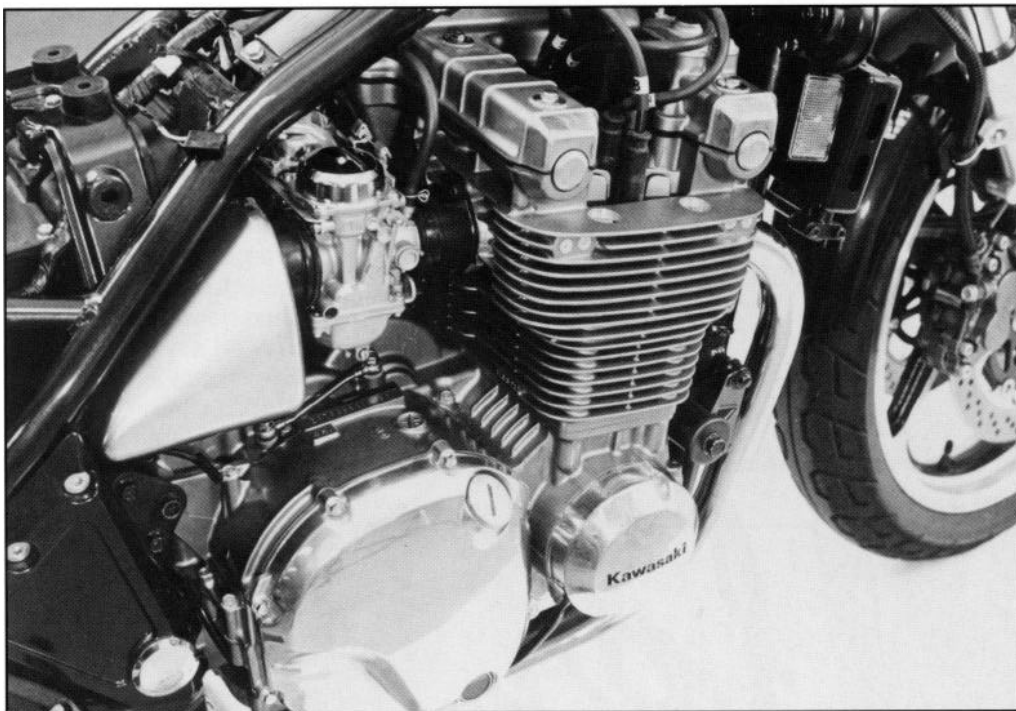
The ZR1100's air-cooled four is all-new, but there's no mistaking its heritage.
