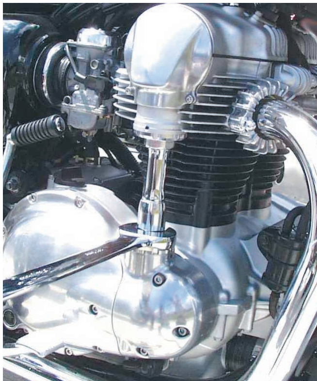
The gear lash of the bevel gear cam drive system can be altered by adjusting the upper or lower (pictured) gear case.
