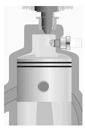
Stratified combustion is used below 5500 RPM. Fuel is ignited just after it leaves the injector with the spark plug firing as many as 15 times to burn fuel more completely.
