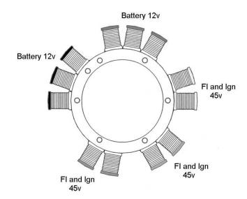
The high output stator has separate coils for a 45-Volt system and a 12-Volt system
