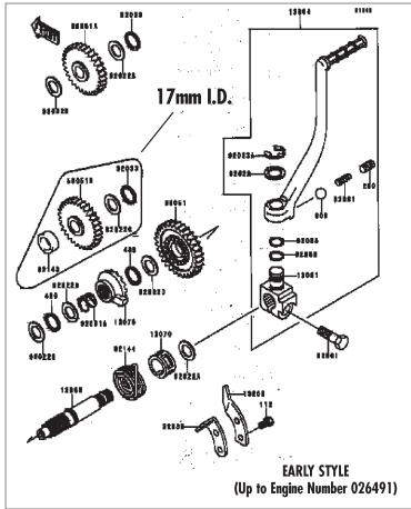
mission shaft where the idler gear rides. The early shaft and gear are 17mm and are used in engine numbers up to 026491. The late parts are 19mm and are used in engine numbers 026492 and up.
