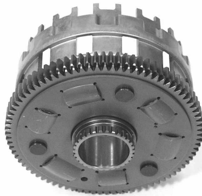
A scissor type primary gear on the ZX-12R eliminates gear lash noise by spring loading the teeth.
