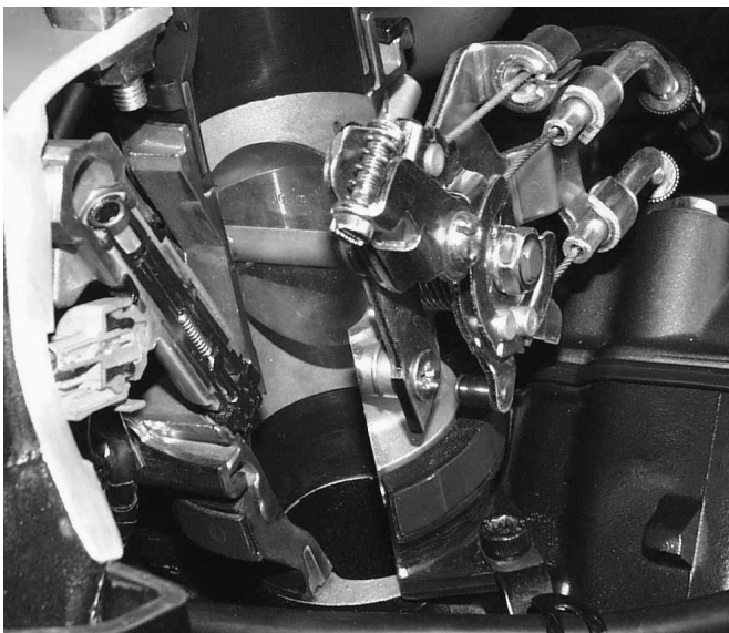
The ZX-12R uses a new Denso fuel injection system.
