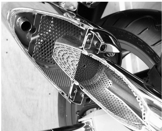
All U.S. model ZX-12R, ZX-9R, and ZX-6R motorcycles come with a catalyzer. All ZX-12R models come with a completely Titanium muffler. CA model ZX-9R and ZX-6R models have dual catalyzers
