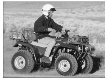
In 1998, Kawasaki offers California model ATVs and KLX300Rs like this Bayou® 220. Carburetor jetting is changed and crankcase vapors are now vented to this airbox.
