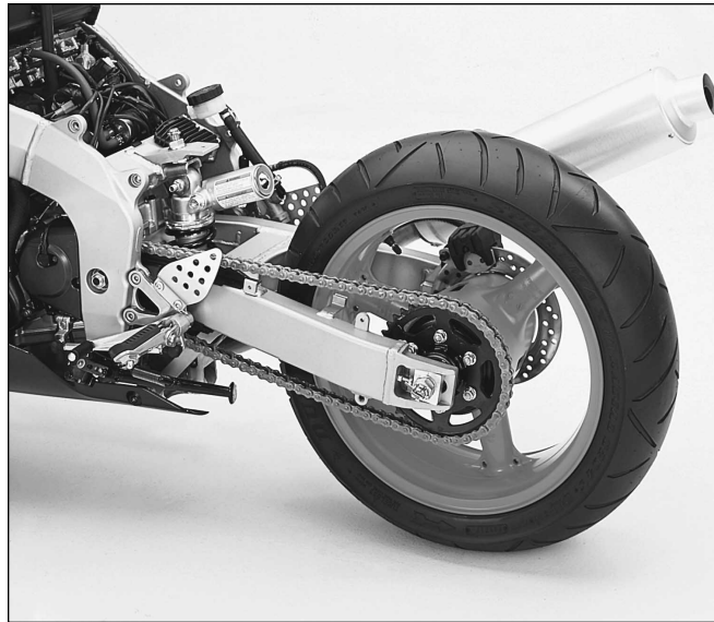
New piggyback reservoir shock for both models. ZX-6R features adjustable ride height, removable subframe, and larger 5.5-inch rear rim.
