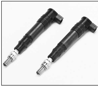
ZX-9R stick type coils are spark plug caps and coils in one.
